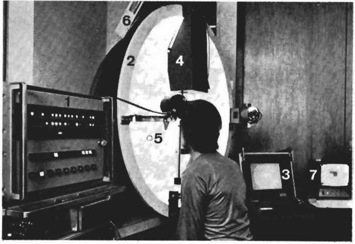
FIGURE 2—Spahr-Fankhauser computer-controlled perimeter including computer, digital magnetic tape, display terminal and eye position monitor. This figure is taken from reference 5 with the permission of the author and publisher.
