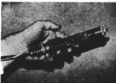
Probe is shown with shield removed
