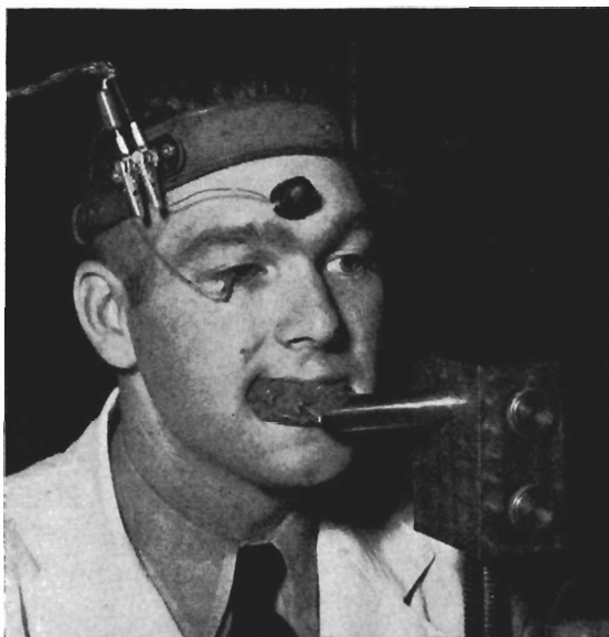
Fig. 4. Subject fixed in position by a dental impression bite, with corneal and remote electrodes in place.
